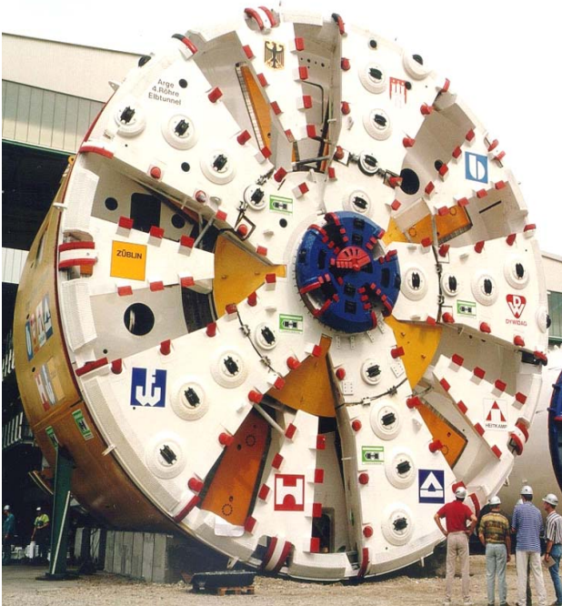
Illus. 1-This Tunnel Boring Machine, with a cutter head measuring approximately 46 feet (14.2 meters) high, was used in a project under the Elbe River at Hamburg, Germany.
