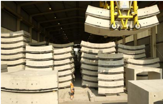
Illus. 2—Sections of the concrete tunnel wall before construction—each section weighs nearly 14 tons
