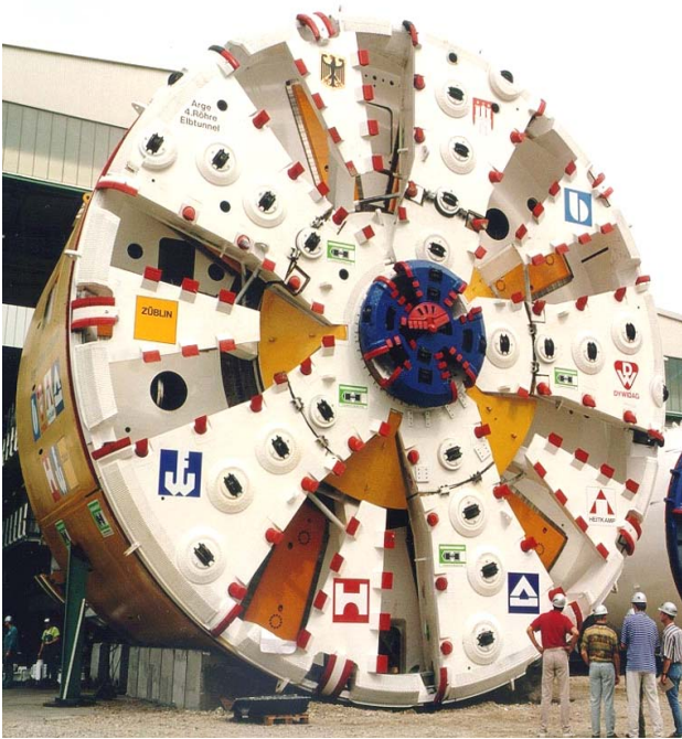
Illus. 1-This Tunnel Boring Machine, with a cutter head measuring approximately 46 feet (14.2 meters) high, was used in a project under the Elbe River at Hamburg, Germany.
