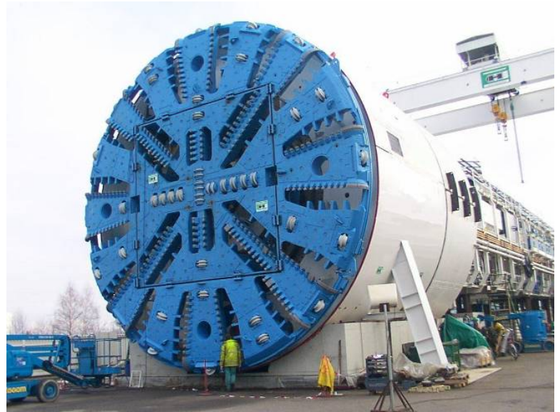
Illus. 2-This Tunnel Boring Machine, measuring approximately 39.5 feet (12.06 meters) high and showing its trailing support gear , was used in a project in Barcelona, Spain.
